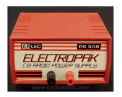
Model: PS 348 Amperes: 1 Price: \$30-up Description: The Electropak was a basic 13.8 volt D.C. power supply, designed for AM CB Radios or low powered <sup>4</sup>
